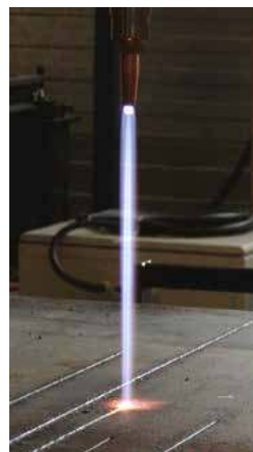
Strong cutting oxygen stream from a divergent nozzle: Photo taken from KOIKE in-house performance test. Nozzle tip at 275 mm above the plate, nozzle 106-D7#0
